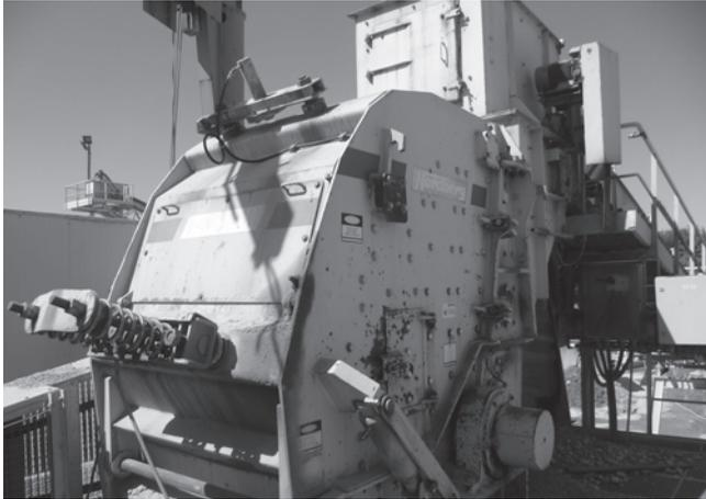
FIG. 6. À LA FIN DU CIRCUIT, LES GRAVATS INERTES PURIFIÉS DES FRACTIONS POLLUANTES PASSENT DANS UN CONCASSEUR AFIN D'OBTENIR DES GRANULATS D'UNE TAILLE DONNÉE. SOURCE : ROTOR ASBL.
